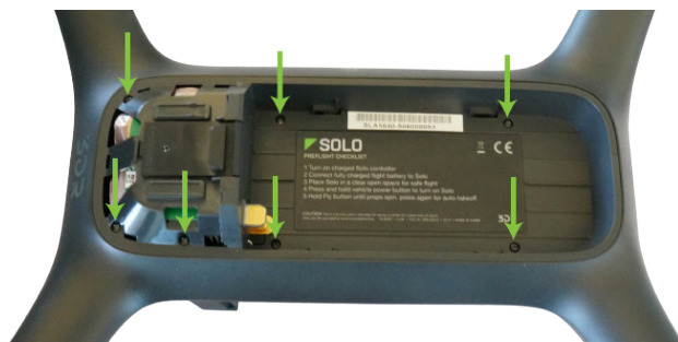
Figure 10.5.2.1: Battery Tray Removal
