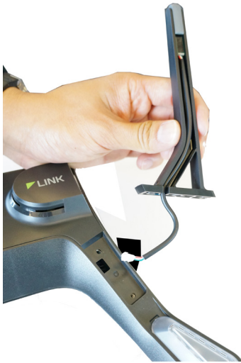
Figure 10.4.3.2: Insert New Leg with Compass
