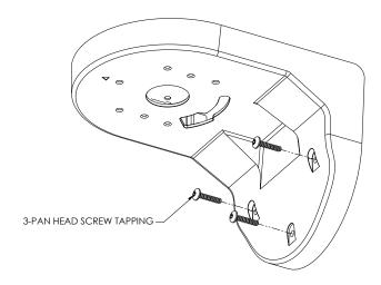
Tighten the plate to wall mount bracket with T4\*20 screws (not to use screws other than flat heads), and connect all necessary cables through the hole on the plate and wall mount kit
