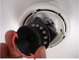
Remove the lens focus tuner.
