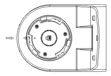
Insert the cables (Network) through the mounting plate and connect to the camera. Then use the little strap in bundled accessory to fasten the network cable.
