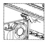
Twist the bracket into place at the back of the installed graphic card. Then install the two included screws to secure the bracket to the drive bay. This will help support the weight of your video card, protecting both the video card and the motherboard.
