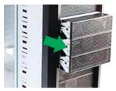
4. If necessary, please remove the HDD cage that is preinstalled in the bay.
