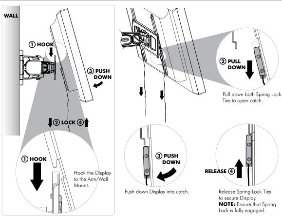
Step 7. Attach Locking Blocks to fully secure the Display
