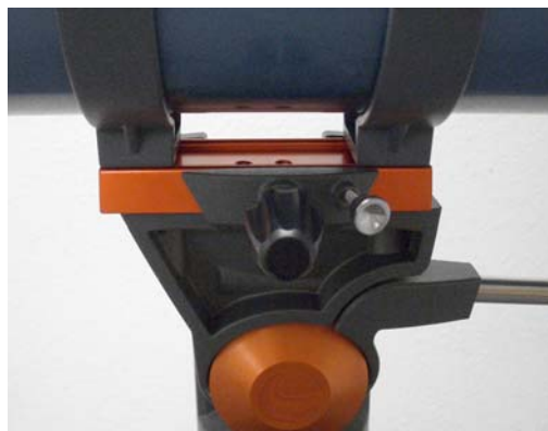
Figure 2-12 Mounting Knob & Safety Screw in the dovetail bracket. Shown is the 90AZ telescope tube
