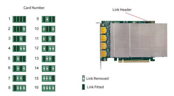
The links control the order in which the display driver uses the ImageDP4+ cards. Knowing the order in which the ImageDP4+ cards are used is useful when connecting the screens and the outputs from video switches.
