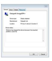
All the cards in your system are driven together to display a single, virtual desktop across multiple screens. Users should be aware that although error code 43 is reported, this is in fact normal operation and there are no faults with the ImageDP4+ cards installed in your system.
