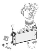
5. Rotate your mobile device to the desired position.
