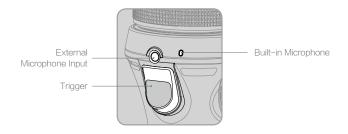
The external microphone will override audio reception of the built-in microphone.
