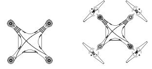
Tighten the propellers with both hands before each flight.
