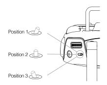
P-mode (Positioning): P-mode works best when the GPS signal is strong. The aircraft utilizes GPS, stereo Vision System to stabilize, avoid obstacles or track moving subjects. Advanced features such as TapFly and ActiveTrack are enabled in this mode.
