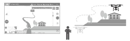
The aircraft will automatically adjust its speed when it senses an obstacle in front or if it is flying too close to the ground. However, this feature should not be relied upon for navigation between obstacles. Failsafe procedures will override Draw. If the GPS signal weakens, the aircraft will exit autonomous flight and return to home.
