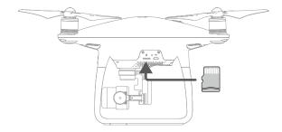
Do not remove the Micro SD card from the Phantom 4 Advanced / Advanced+ when it is shooting.
