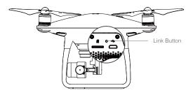
The remote controller will un-link itself from an aircraft if a new remote controller is linked to the same aircraft.
