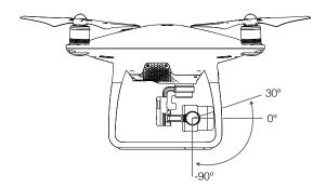
Use the gimbal dial on the remote controller to control the tilt movement of the camera.
