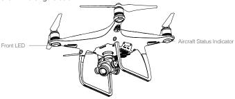
The Front LEDs show the orientation of the aircraft. The Front LEDs glow solid red when the aircraft is turned on to indicate the front (or nose) of the aircraft. The Aircraft Status Indicators communicate the system status of the flight controller. Refer to the table below for more information about the Aircraft Status Indicators.
