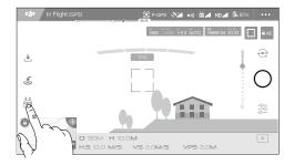
3. Tap once on the target direction and wait for icon to appear. Tap again to confirm the selection and the aircraft will automatically fly towards the target direction.
