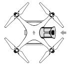
Make sure that you hear a click sound indicates the battery is firmly installed. Failure to do so may affect the flight safety of your aircraft.
