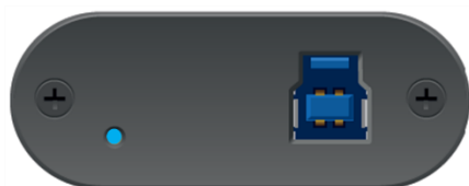
A solid blue LED means USB 3.0
