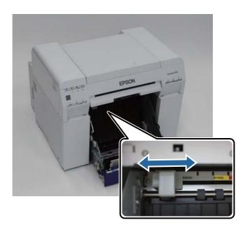
2 Load the spindle unit in the roll paper feeder with gray adapter on the left.
