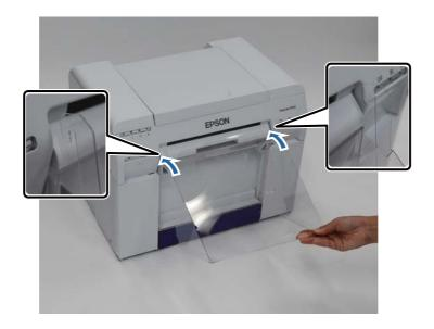
When the length of the print size is 3.5 to 4 inches (89 to 102 mm), place the hooks into the top holes. When the length of the print size is 4 to 8 inches (102 to 203 mm), place the hooks into the bottom holes.
