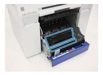
Use a piece of masking tape to remove any dust from the pickup rollers. Rotate the rollers and repeat the process as necessary until you've removed all of the dust.
