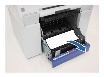
Lower the front place and press down until you hear it click into place. Repeat this for the rear plate.
