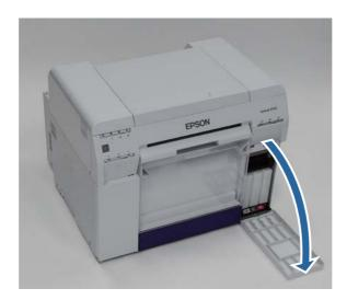
Push up on the maintenance tank, then carefully remove it. Make sure not to tilt the cartridge.
