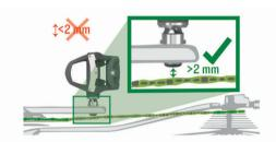
**NOTE:** Garmin recommends 2 mm or more between the pedal and the chain. If the pedal rubs the chain, you can add one washer (included) between the spindle and the crank arm to increase clearance. To maintain an equal q factor, you can add one washer to the left pedal spindle. Do not use more than one washer on each pedal.
