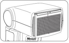
• For portrait photography, pull out the light diffusing panel and place it over the flash window as shown in the picture. The diffusing panel makes the flash light soften and creates a lively color effect on the subject.
