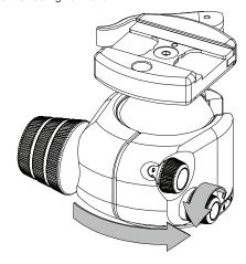
2. Fully seat camera into the drop notch.
