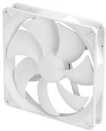
FM181 180mm fan with variable speed controller, fan speed ranges from 500rpm to 1300rpm (65CFM to 150CFM)
