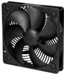
AP181 Air Penetrator AP181 180mm fan, dual speeds at 700rpm and 1200rpm (80/130CFM)
