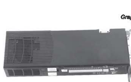
Graphics card with backplate photo (9800GX2)
