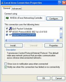
4. Select "Use the following IP address", and type in *IP address : 192.168.2.100*
