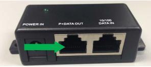
6. Using another Ethernet cable, connect one end to the **DATA IN** port of the injector.
