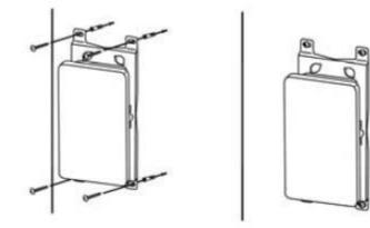
Position the provided mounting bracket to the desired location and mount as shown in the above image using the provided wood screws and plugs.
