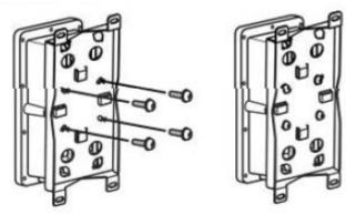
Align the mounting triangle to the back of the access point. Securely tighten the mounting triangle by using the M5x10 screws and washers.
