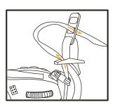
2. Then, thread the hand grip strap through the adjustment buckle that is facing the camera, loop the strap over and thread through the bottom shoulder strap mount. The remaining strap will thread through the opposing side of the adjustment buckle.
