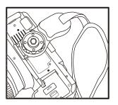
4. Align the 1/4"-20 thumb screw plate with the camera's tripod mount and begin to tighten.
