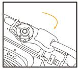
5. Rotate the 1/4"-20 thumb screw plate while securely tightening the 1/4"-20 thumb screw, and ensure that the thumb screw plate tab is properly aligned with the camera's base.
