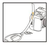
1. Thread the hand grip strap through the strap mount on the camera.
