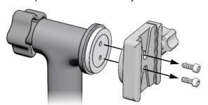
**Tip:** Keep the clamp and extra screws handy so that you can convert the Head back to the Sidemount when shooting conditions require a lighter, more compact set up.
