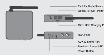
\*In SPDIF mode, connect devices through SPDIF IN for TX mode and SPDIF OUT for RX mode
