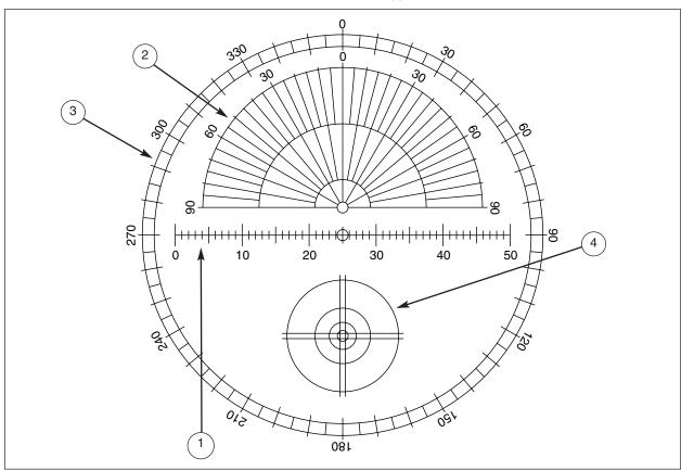
**Fig. 2:** MA 12mm Astrometric Eyepiece Reticle. (1) Linear Diameter Scale, (2) Semicircular Position Angle Scale; (3) 360° Position Angle Scale; (4) Double Crossline/Concentric Circle Guiding Scale.
