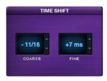
**Time Shift** allows Grooves to be offset by a number of beats (Coarse), or shifted in time (Fine):
