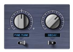
The knobs on the **Easy Edit Page** are dual mode controls. Clicking the switches below each knob alternates between modes.
