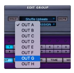
This window allows you to route the audio of an Edit Group to any of the eight stereo audio outputs (if your host supports it). This output assignment is pre-mixer, so the audio will not be affected if Outs B-H are chosen on the Mixer page. Clicking on the window itself reveals a drop-down menu with all available Outputs. This feature makes it easy to process and route selected pieces of audio outside RMX if desired.
