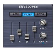
There are three independent Envelope generators – **AMP**, **FILTER**, and **PITCH**. Each Envelope has its own sub-page with a set of dedicated controls. To activate a sub-page, click one of the three names. These **Envelopes** work on a per-slice basis.
