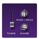
The Timing section of the Chaos Designer subtly affects the playback timing of slices in relation to their original starting positions in the rhythm. This is similar to the "humanizing" function found in many sequencers, but applied to audio loops. There are three parameters in this section that determine how much and what kinds of changes will occur. Imagine Zero on these sliders as being "Never," maximum being "Always," and in-between the two extremes are increasing ranges of "Sometimes."
