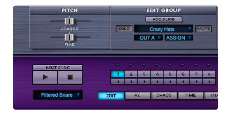
The **SLICE EDIT GROUP** option in the Footer's Value Display can be a big help while using ADD / REMOVE. Switching to this mode allows you to see the Edit Group membership of the currently played Slice.
