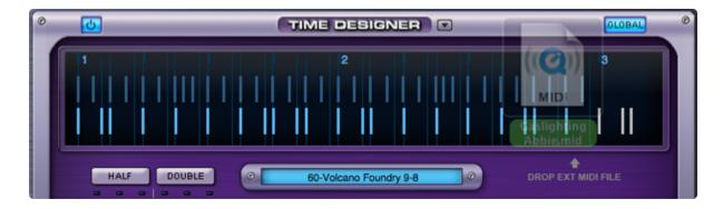
NOTE: Importing an external MIDI file when the <u>Global Button</u> is enabled will apply the MIDI file's feel to all the Parts in the Multi.
