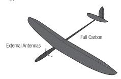
Slide the feeder antennas through the holes until the 31mm tip, and about 2mm of coaxial, completely exit the fuselage. Use a drop of CA or tape to fix the antenna to the fuselage.
