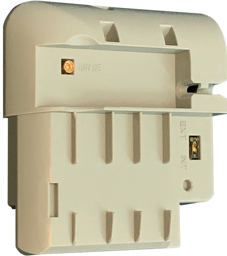
Figure D.1: A Cellular Module
