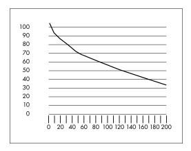
The curve can be applied to any lead acid battery under load providing that it has an AH rating at the 20 hour rate.
